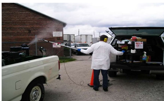
Clarke Mosquito Control checking droplet size
